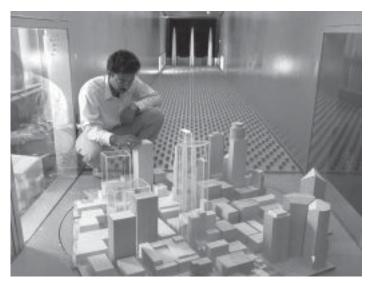
A model of downtown Minneapolis is prepared for testing in the boundary layer wind tunnel at the University of Minnesota's St. Anthony Falls Laboratory (SAFL). The test will study the effects of wind on structures. The SAFL was recently awarded a Science and Technology Center award. Courtesy Pat Swanson, St. Anthony Falls Laboratory, Univ. of Minnesota.
